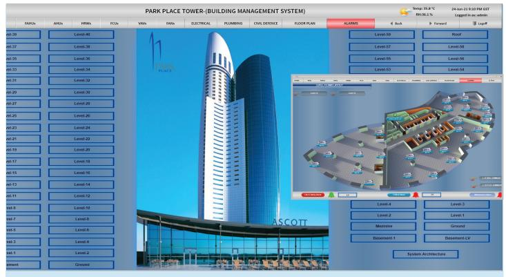
The customized user interface built for the Park Place Tower features a graphical navigation system that allows the facilities management team to easily visualize the status of building services in the tower at the whole-building, floor, equipment and VAV levels. This makes the root cause of alarms easy to trace, and it speeds response time. The facility team is empowered to monitor trends and address issues before comfort and energy use is impacted.
