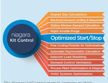
The Niagara kitControl module contains multiple easy-to-use logic blocks for proven energy saving and optimization strategies. The Conti team used the Optimized Start-Stop block to set parameters informed by desired space conditions and area characteristics. The algorithm then calculates an optimal amount of lead-time before a scheduled event.
