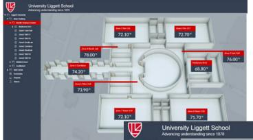
The UI developed by Conti with Niagara Workbench offers easily interpretable information starting with this heat-map view of a whole building. The visual temperature indication allows the ULS team to quickly determine any problem units and take fast action.
